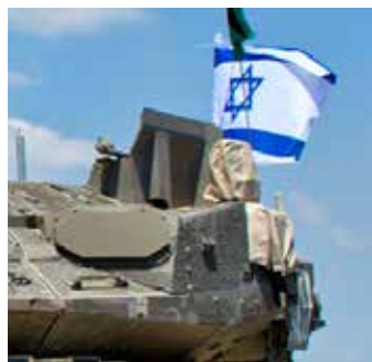
Rafael's Trophy Active Protection System on an Israeli Merkava battle tank. The U.S. purchased APS last June for use on about 250 of its own M1 Abrams Tanks.
