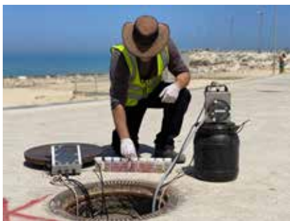
The Kando system gathers samples that are taken to a lab for virus testing.
